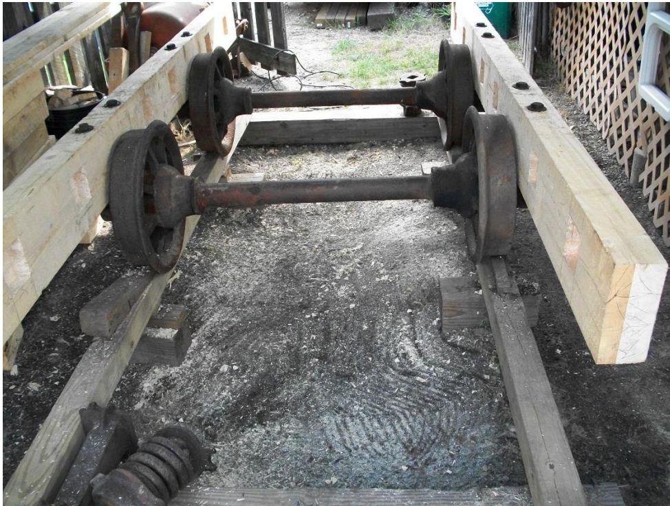
5- Bolting side beams to journals
